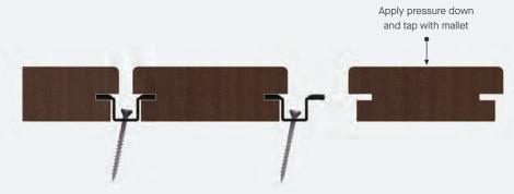
Pre-cutting and loose laying 5-10+ rows in advance is the most effective way of working. This allows you to oil the backs of the boards (pre-oiling will save oiling the back of the board) prior to laying and to see where to install double clips for butt joins in advance.
